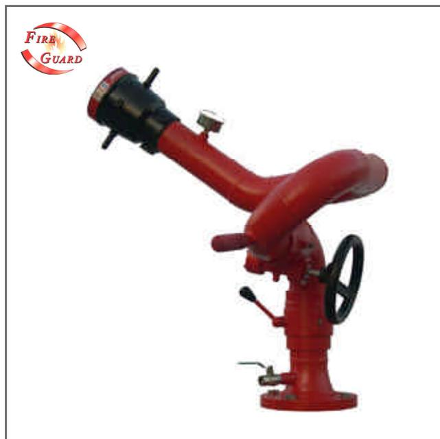
resistant bronze swiveling joints with double row of stainless steel ball bearing. Vertical movement is controlled with single handwheel driven enclosed worm gear and twist lock for horizontal movement.
