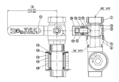
Fireguard TESTANDRAIN is a 300 PSI rated single handle ball valve that was specifically designed to provide both the test function and the express drain function required for a wet fire sprinkler system. It features a tamper resistant test orifice, integral tamper resistant sight glasses, and a tapped port for system access. Fireguard TESTANDRAIN meets all the requirements of NFPA-13, NFPA-13R, and NFPA-13D. Available in 1", 1-1/4" and 2" sizes in both NPT and BSPT
