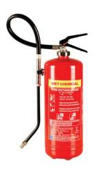
Wet chemical Fire extinguishers are the new innovation for cooking fat fires. Wet chemical is the most effective means for extinguishing fires involving deep fat friers. The solution cools and emulsifies when applied to burning fats and oils.
